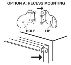
A. RECESS MOUNTING: Mounting to the inside of the window frame.
