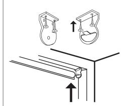
C. TOP MOUNTING: Mounting overhead to the top inside of the window frame or the ceiling.
