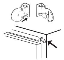
B. FACE MOUNTING: Mounting to the outside of the window frame.
