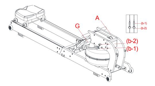
6. With the tool (84), remove the screw #61 that is pre-locked on the main frame (A). With the tool (84) as shown, remove the screw #61 that is just removed and lock the electronic watch assembly (G) and the main frame (A) together.
