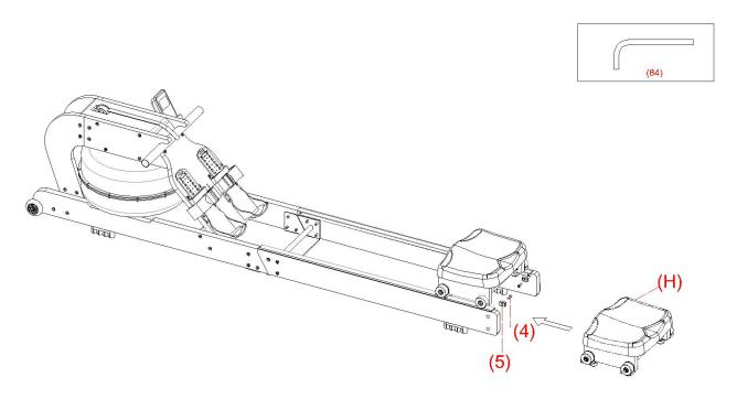
3. Remove 2 hexagonal cylindrical head screws (4) and 2 cushion blocks (5) placed on one side and lock them back to the left and right slide rails using a tool (84).
