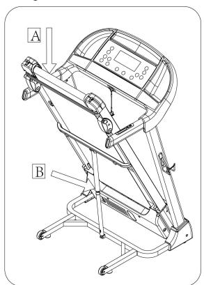
Support place A with hand, kick the place of air pressure bar, then the base frame will fall down automatically (Please keep anybody and any pet away the machine when falling down).
