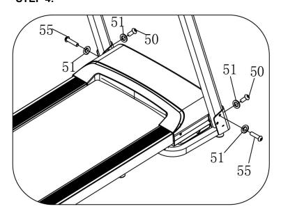
1.Use 5# Allen wrench, firstly lock upright onto base frame by bolt (55) and lock washer (51), then lock upright onto base frame by bolt (50) and lock washer (51).
